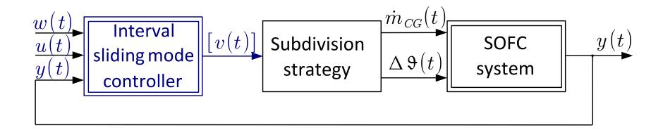
• Mathematical model of the SOFC system in an input-affine description is extended by a bounded disturbance  $d \in [d]$
