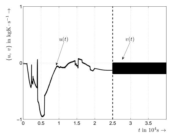
**Problem:** Adequate setting of the SOFC system input  $u = \dot{m}_{CG} \Delta \vartheta$  with an available sliding mode controller output v(t)
