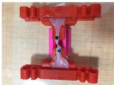
Ruptured sample after the experiment.
