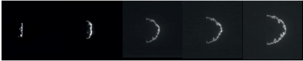
Fig. 2. Propagation of a diffracting detonation wave with subsequent attenuation.
