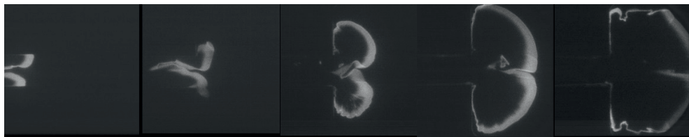
Fig. 1. Propagation of the flame front followed by diffraction.
